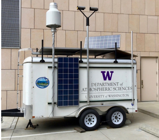
The UW Atmospheric Sciences Building Weather Station that is monitoring and transmitting data to a web portal
