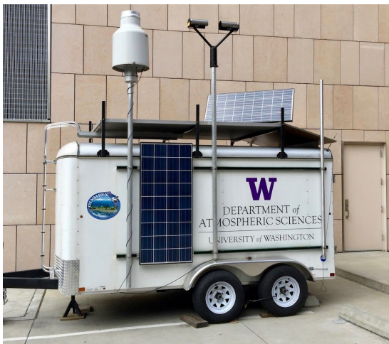
The UW Atmospheric Sciences Building Weather Station that is monitoring and transmitting data to a web portal
